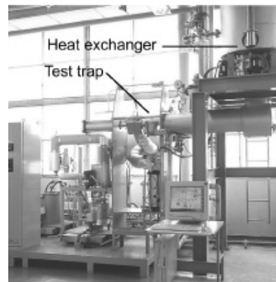
Figure 5: ISO 7841 test rig at TLV Co Ltd
