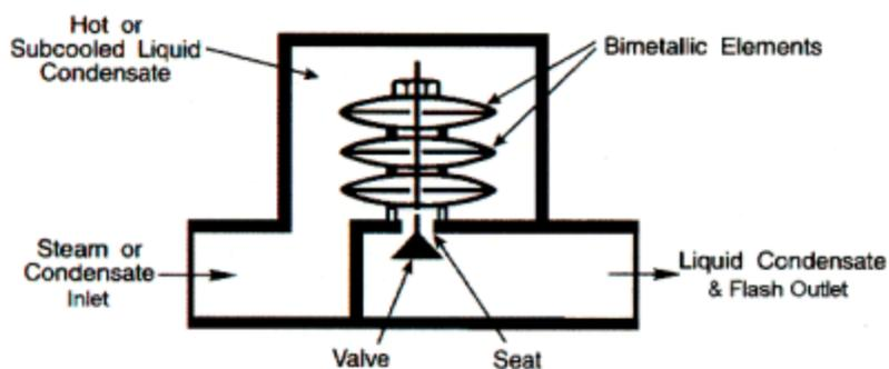
**Figure 2. Bimetallic steam trap.**
