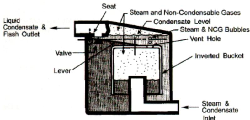
**Figure 1. Inverted bucket steam trap.**
