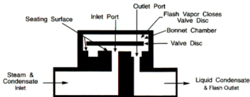
**Figure 5. Disc steam trap.**
